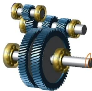
Figure 4.4 Two-stage helical gear transmission developed by AVL
