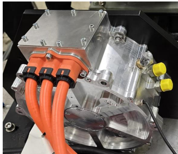
Figure 4.2 TRX axial flux motor featuring a yokeless, dual-rotor single-stator design.
